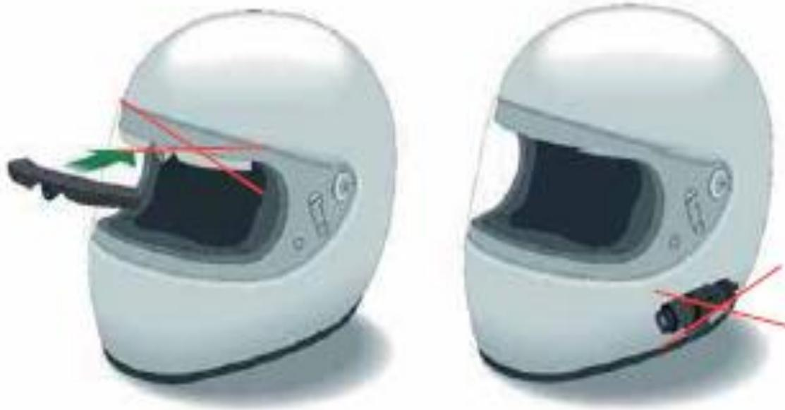
*Fig.1 – NOT approved helmet camera installation*
